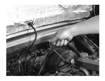
2. Insert the Extracting tube into the dipstick hole until it reaches the bottom of oil pan. connect the Main Suction Tube into the Fluid Inlet Coupler with Main Suction Tube Adapter.
